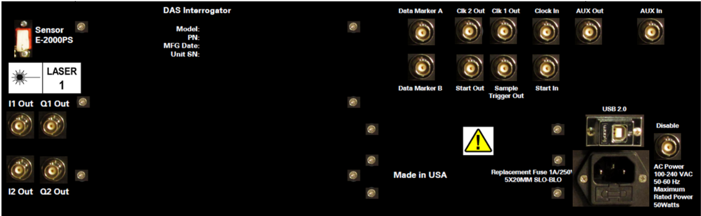
Optical E-2000PS to sensor (1), USB Control Interface (1), Signal Out shown for DP1 (4), Two quadrature pairs I & Q Data Markers In (2), Used for GPS time stamp or test tones Sample Trigger Out (1), DAQ trigger for data frame Clk In/Out, Aux In/Out, Start In/Out (5), Used to synchronize to Host DAQ or other DAS interrogators Safety Interlock In (1)
